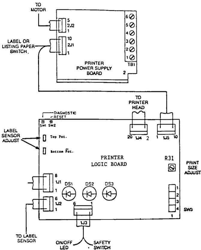
FIG. 2 Hobart 18VP Thermal Printer,<sup>2</sup> Circuit Boards
