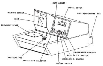
FIG. 2 Clearwave Optical Character Tester (082)<sup>2</sup>
