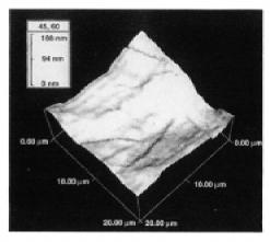
FIG. 9 Stainless Steel Surfaces Used for SA Index,  $Z_{max}$ , and  $Z_{rms}$  Data Given in Table 1
