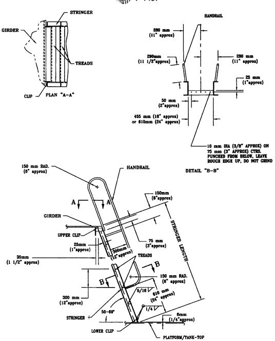
FIG. 1 Type I Ladder Elevation
