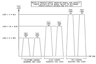
FIG. 6 APD Acoustic Emission Test Sequence
