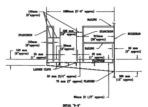
FIG. 2 Cargo Platform Elevation
