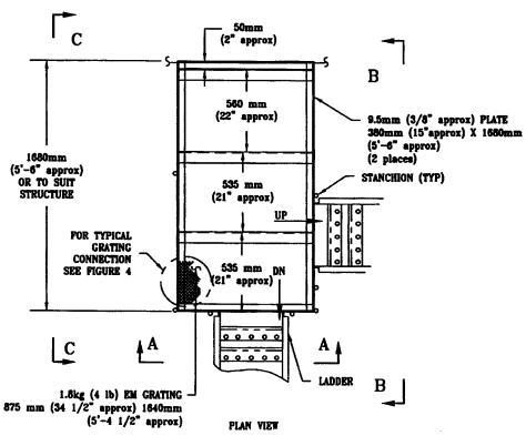
FIG. 1 Cargo Platform—Bulkhead
