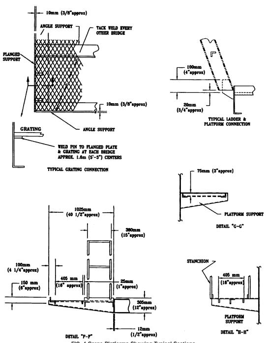
FIG. 4 Cargo Platforms Showing Typical Sections
