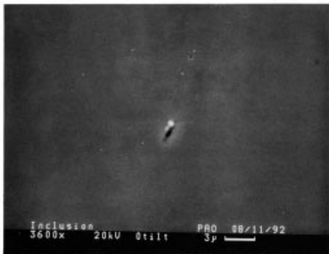
FIG. 2 Example of Pit Defect (3600 × magnification)
