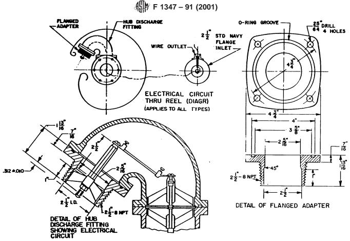
FIG. 2 Discharge Fitting and Adapter Details for Type 1 and 3, 2<sup>1</sup>/<sub>2</sub>-in. (65-mm) Collapsible Reels
