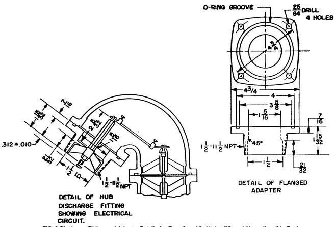
FIG. 3 Discharge Fitting and Adapter Details for Type 2 and 3, 1<sup>1</sup>/<sub>2</sub>-in. (38-mm) Noncollapsible Reels
