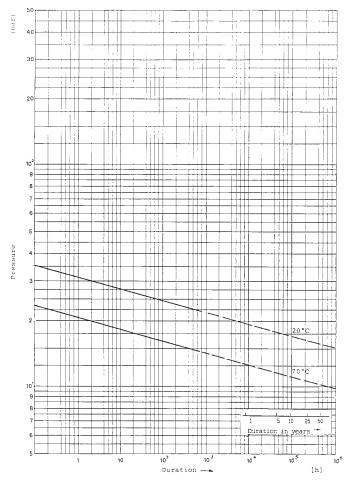
NOTE 1—The reading of the graphs indicates the pressure rating applicable to the different classes of pipe. This takes into account the temperature of utilization and the desired duration of use.
