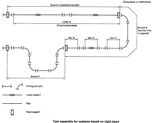
FIG. 8 Hot and Cold Pressure Cycling Test
