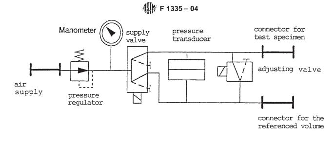
Test bed example for vacuum depression test FIG.7 Vacuum Depression Test
