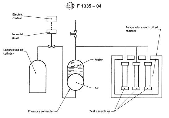
Diagram of typical equipment arrangement for cyclic pressure shock test FIG. 9 Water Hammer Test
