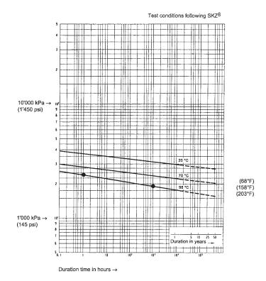
NOTE—The reading of the graph indicates the pressure rating applicable to the two classes of pipe. This takes into account the temperature of utilization and the desired duration of use.
