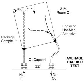
FIG. 3 Attachment Method for Flexible Pouches
