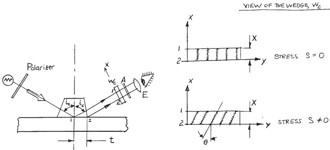
FIG. 1 Apparatus For Measuring Surface Stress
