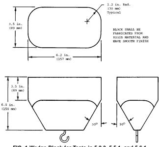
FIG. 1 Wedge Block for Tests in 5.2.3, 5.5.1, and 5.6.1
