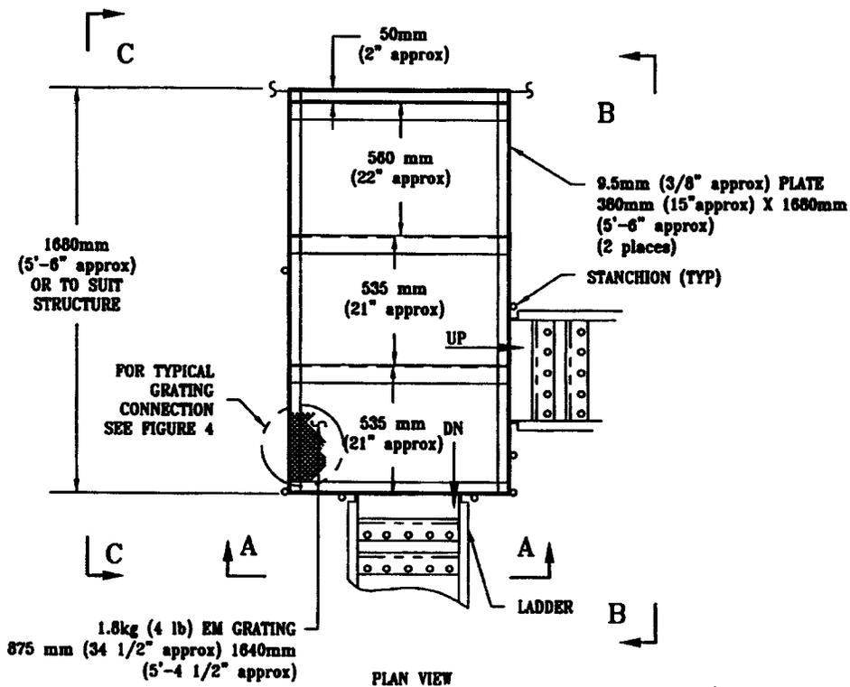
FIG. 1 Cargo Platform—Bulkhead
