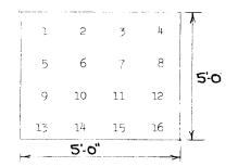
FIG. 3 Location of Wet-Film Thickness Readings
