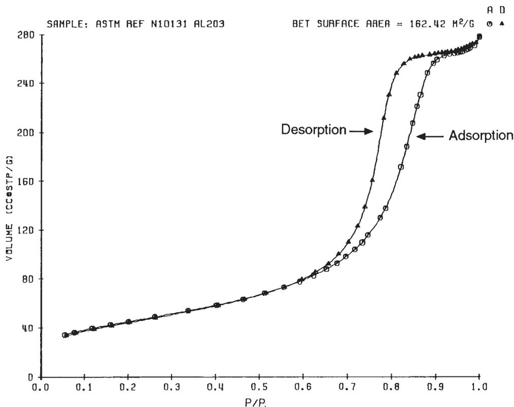
FIG. 2 Adsorption-Desorption Isotherms
