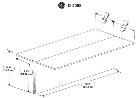
FIG. 1 Bonded-Seam T-Peel Sample After Bonding and Prior to Specimen Cutting and Selection
