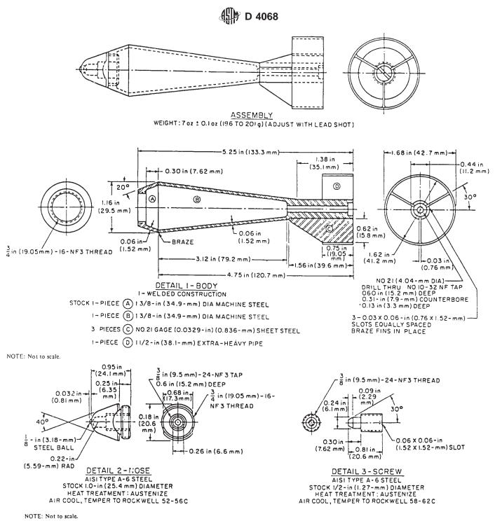
FIG. A3.2 Dart for Safety Glass Tests
