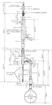
FIG. 1 Distillation Apparatus
