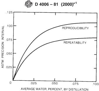
FIG. 3 Basic Sediment and Water Precision
