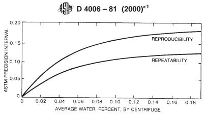
FIG. X1.2 Basic Sediment and Water Precision for ASTM Test Method D 1796 Centrifuge Method (Based on Five Laboratories)
