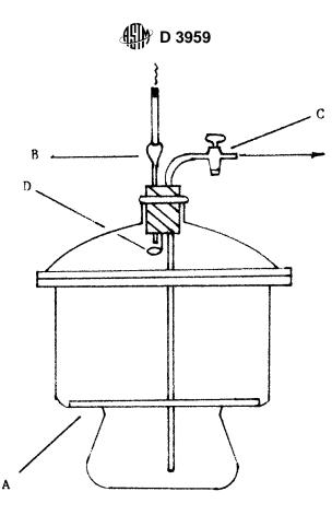
A-Glass plate with attached specimens
