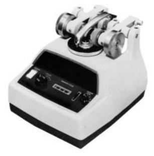
FIG. 1 Rotary Platform Double Head Abrader
