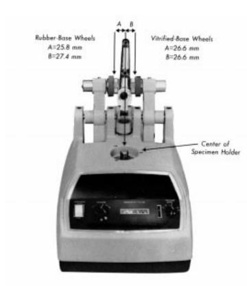
FIG. 2 Position of Abrasive Wheels on Rotary Platform Double Head Abrader
