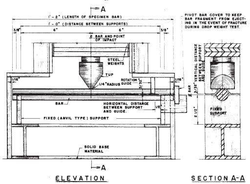
FIG. 2 Typical Example of Drop-Weight Test Apparatus
