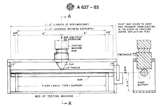
FIG. 4 Typical Example of Deflection Test Apparatus
