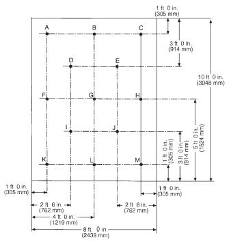
FIG. 2 Dowel Placement in Chamber Floor
