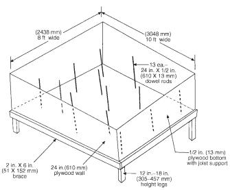
FIG. 1 Installed Thickness Test Chamber
