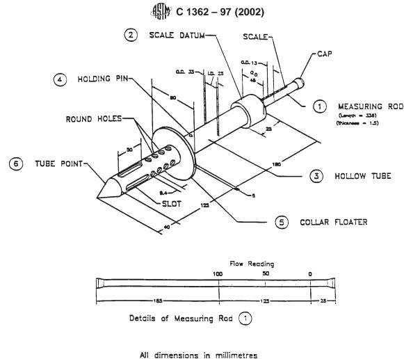
(1 in. = 25.4 mm) FIG. 1 Apparatus for Flow Test
