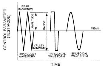
FIG. 1 Cyclic Fatigue Nomenclature and Wave Forms
