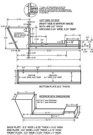
END PLATE - 6.5° WIDE X 0.25° THICK X 4.75° HIGH FRONT PLATE - 6.5° WIDE X 0.25° THICK X 1° HIGH GATE PLATE - 6.5° WIDE X 0.25° THICK X 1° HIGH COVER PLATE - 6.5° WIDE X 0.25° THICK X 1° HIGH COVER PLATE - 6.5° WIDE X 0.25° THICK X 2° HIGH (FOR 2° POUR THICKNESS), X 2.75° HIGH (FOR 1° POUR THICKNESS),
