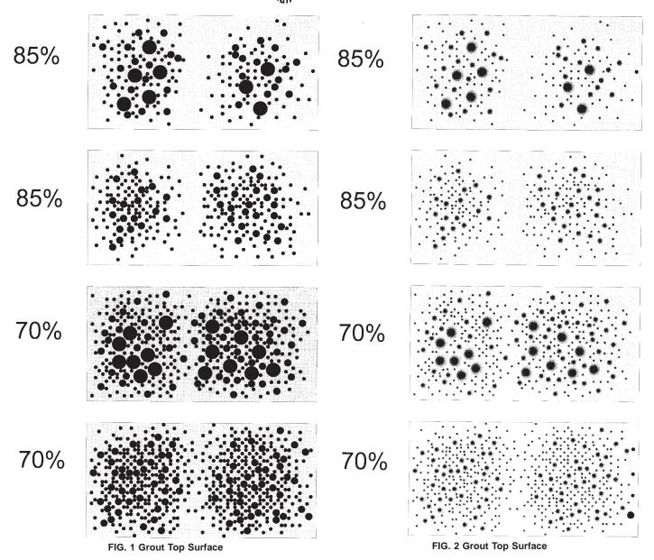
5.5 The estimated amount of upper grout surface contact in percent can be used to compare two or more grouts or show the effects of temperature, formulation changes, or other factors on bearing area. Because of the limited accuracy in estimating the percent of contact, a limited set of results is suggested (see 9.9.1). Visual guides are provided for comparative purposes (see Fig. 1 and Fig. 2).
