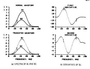
Note 1—The truncated version of the spectrum of  $B_2$  in (a) is used to obtain the first and second derivatives in (b). The derivatives are used as indicated by the vertical markers to define the "valid zone" or usable frequency range.
