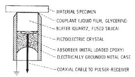
FIG. 1 Cross Section of Buffered Broadband Ultrasonic Probe
