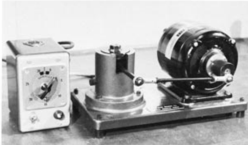
FIG. 1 Fafnir Friction Oxidation Tester and Time Switch
