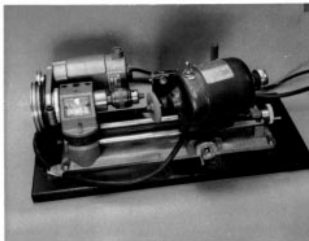
FIG. 1 Machine Setup for Needle Sharpening
